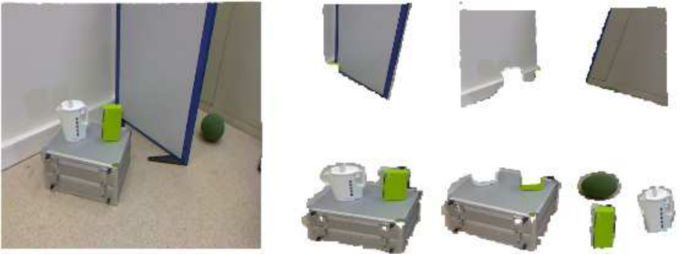
Fig. 3. Example of the segmentation with the baseline system. Left: original point cloud after re-sampling. Right (upper row): detected walls which are subsequently removed. Right (lower row): Segmented objects including objects placed on top of each other. The whole group is segmented as a single object at first. Detection of the horizontal plane on the metal suitcase allows to separate the suitcase from the three objects placed on top of it.
