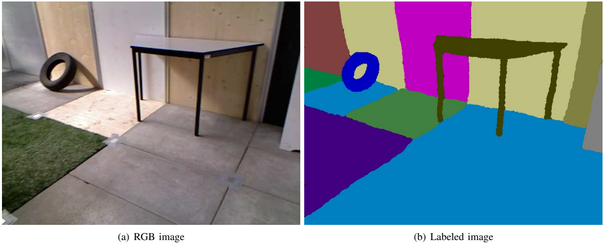
Fig. 2. Examples of image annotations in the PACOM RGBD segmentation database. (a): Original image. (b): annotated image. Each pixel has an identity associated to it, where different pixel colors indicate different identities.
