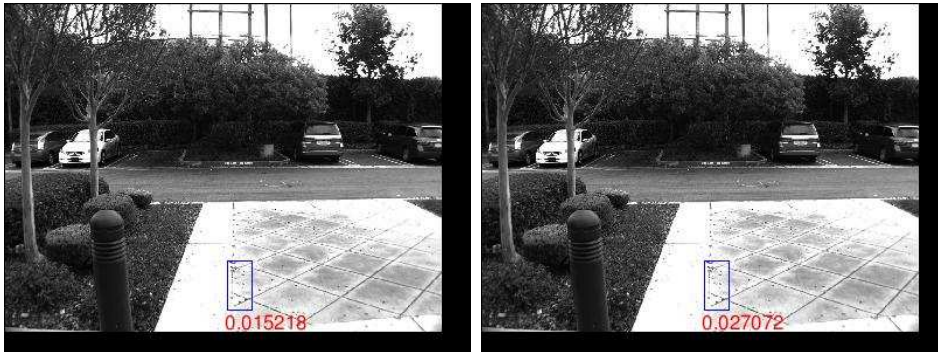
Figure 10: A particular situation where DAPs can actually increase the number of incorrect detections. Shown are two consecutive images from stream 5, see Tab. 3, where an incorrect detection occurs in a spatiotemporally consistent way (non-linear SVM score is shown along with the detection). This will lead to self-enhancement, and therefore to further detections and further tracking. Such undesirable behavior will continue as long as there is a sufficient frequency of incorrect but consistent detections to allow tracking to continue.
